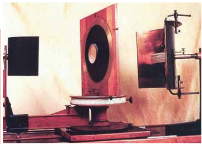
Fig. 3 Righi's Bench for electromagnetic waves, 1893 (Museum of Physics). An educational and experimental device shown by Righi to his university pupils; Marconi was among them.
