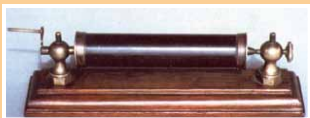
Fig.1 Coherer ( tubetto a limatura ) by T. Calzecchi Onesti (Calzecchi Onesti Family courtesy).
