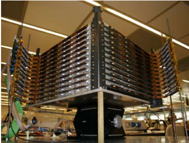
Fig. 3 The AGILE silicon-tungsten tracker during the final assembly and test phase in the INFN laboratories of Trieste and MIPOT facility (June 2005).
