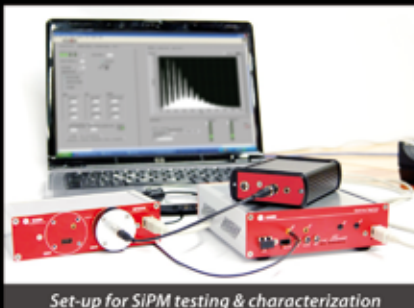
Set-up for SiPM testing & characterization
