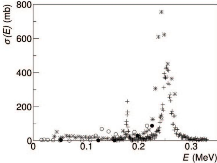
Fig. 1. – Directly measured cross-section data of the two-body  $^{17}\text{O}(n, \alpha)^{14}\text{C}$  reaction as available in the literature. Asterisks are from the data of Sanders [6], circles are from Koehler *et al.* [7], full dots are from Shatz *et al.* [8], crosses are from Wagemans *et al.* [9].
