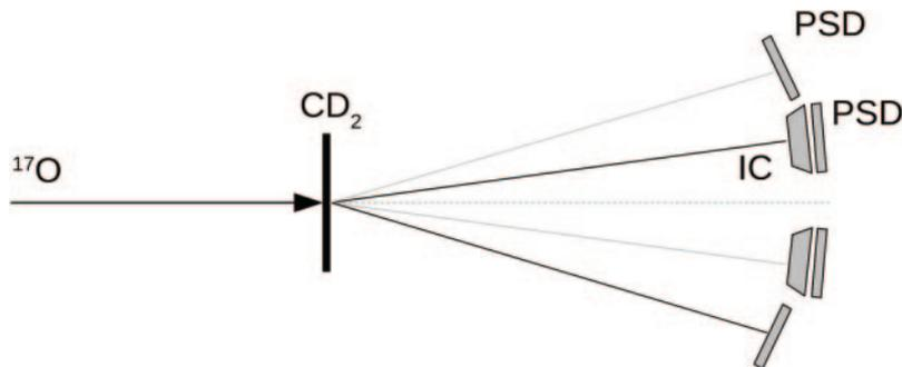
Fig. 2. – Sketch of the experimental setup, not in scale. The  $^{17}\text{O}$  beam was impinging on a  $\text{CD}_2$  target. The emitted particles were detected by two groups of detectors composed of one position sensitive device (PSD) for the  $\alpha$  particles and a  $\Delta E$ - $E$  telescope, made up by an ionization chamber (IC) and another PSD, for the C nuclei.
