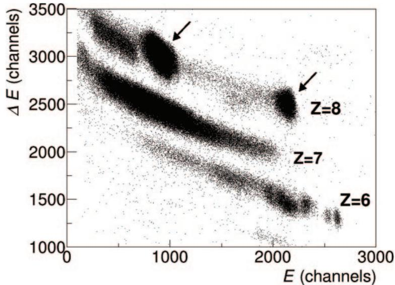
Fig. 3. – Energy loss  $\Delta E$  in the first stage of the telescope plotted against the energy loss  $E$  in the second stage. The black arrows point to the bulges coming from the scattering of the beam on both  $^{12}\text{C}$  (left arrow) and  $^2\text{H}$  (right arrow) nuclei in the  $\text{CD}_2$  target. Adapted from ref. [34].
