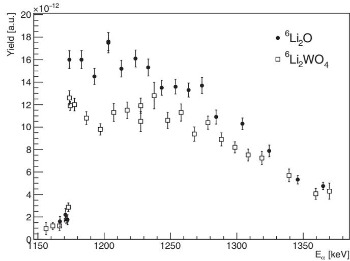
Fig. 4. – Scans of the  ${}^6\text{Li}(\alpha, \gamma){}^{10}\text{B}$  resonance at 1175 keV performed on two different targets used for the measurement of the  ${}^6\text{Li}+p$  cross-section at LUNA.
