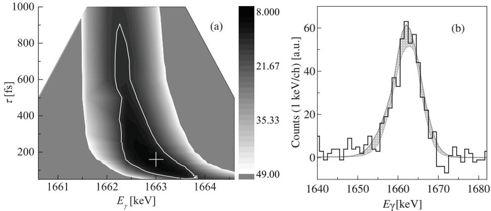
Fig. 6. – (a) Lifetime-energy  $\chi^2$  minimisation surface for the  $^{18}\text{N}$  1663-keV transition. The minimum is indicated by the white cross, while the solid white contour delimits the  $1\sigma$  region. (b) Comparison between the background-subtracted experimental data (black histogram) and the simulated ones within  $1\sigma$  (grey band) for the same 1663-keV transition considered in panel (a).
