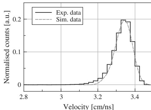
Fig. 1. – Experimentally measured (black histogram) and simulated (dashed line) velocity distribution of the  $^{17}\text{O}$  reaction fragments, considering the population of the  $1/2_1^-$  state at 3055.36(16) keV [12] which decays via the emission of a gamma ray of 2184.44(9) keV [13].
