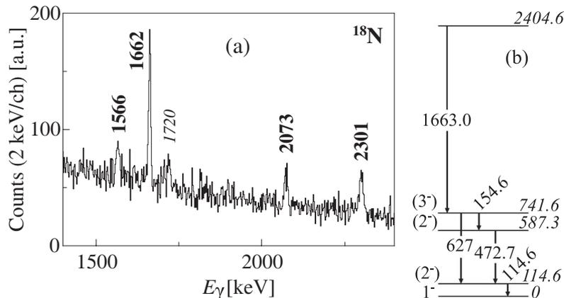
Fig. 5. – (a) Partial AGATA Doppler-corrected  $^{18}\text{N}$   $\gamma$ -ray energy spectrum: the transitions in bold are assigned to the nucleus, while the 1720-keV peak (in italics) assignment is not certain due to limited statistics. (b) Updated version of the  $^{18}\text{N}$  nucleus level scheme of ref. [23], considering lifetime effects (see text for details and error bars).
