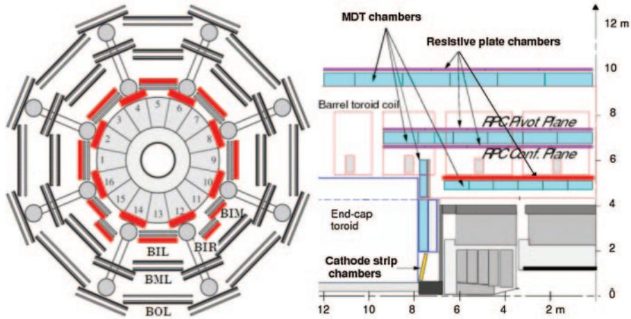
Fig. 1. – Layout of the BI layer in the  $X$ - $Y$  (left) and  $Y$ - $Z$  (right) projections respectively, with the new RPC and sMDT chamber positions indicated in red.
