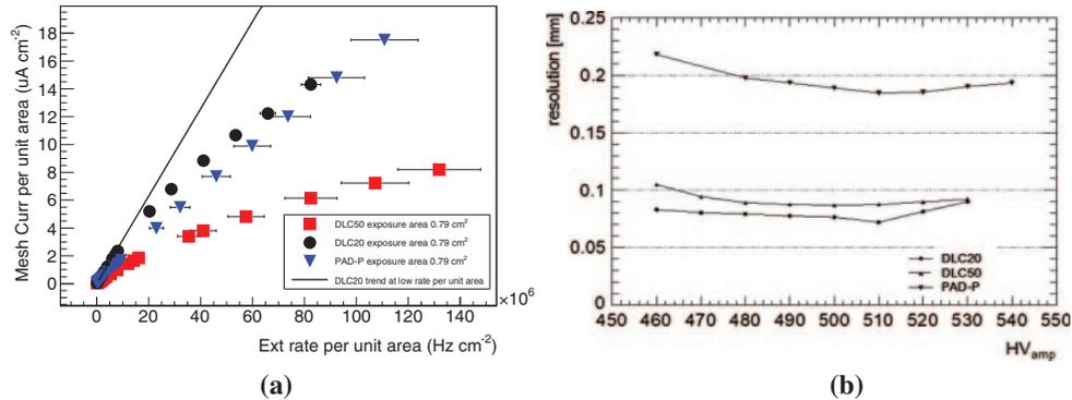
Fig. 1. – Mesh current per unit area as a function of rate per unit area (left) and spatial resolution as a function of amplification voltage (right).
