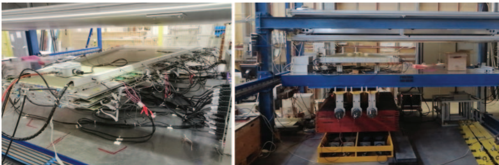
Fig. 8. – Pictures of the Cosmic Ray Stand of the Frascati INFN National Laboratories. Two scintillator planes are used as trigger and are located below the chamber under test.
