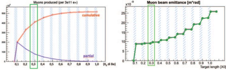
Fig. 6. – Left: muon pairs produced as a function of the target length (in orange the total number of muons produced from the start of the target, in purple the muons produced in that  $0.1X_0$  long slice). Right: emittance of the produced muon beam as a function of the target length, in green the horizontal and in magenta the vertical emittance (not clearly visible because behind the green line).
