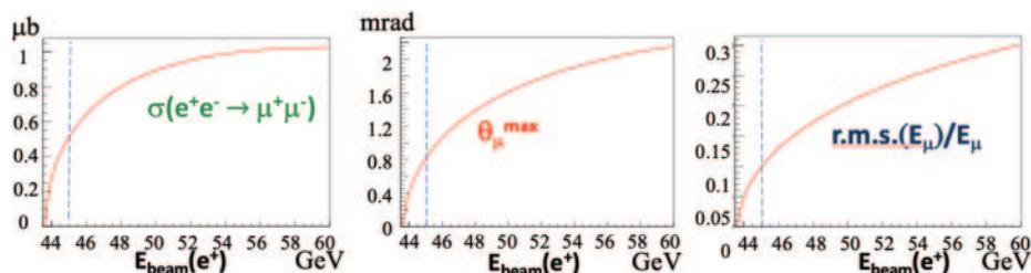
Fig. 5. – Muon production cross-section (left), divergence (center) and energy spread (right) of the produced muons as a function of the positron beam energy.
