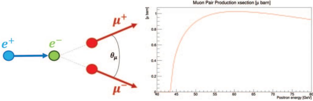
Fig. 1. – Left: schematic of the muon pair production reaction. Right: cross-section of muon production via electron-positron annihilation as a function of the energy of the positron beam.
