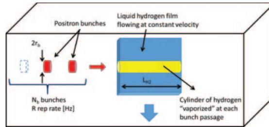
Fig. 8. – Scheme of the liquid target cell.
