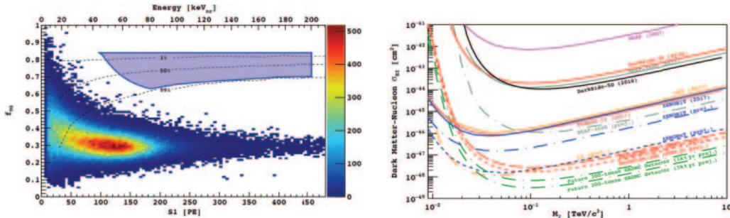
Fig. 2. – On the left, the WIMP search box in the S1 *vs.*  $f_{90}$  region after all the cuts is shown. On the right, the black curve represents the DarkSide-50 90% CL limit on the spin-independent cross-section between WIMP and nucleons.
