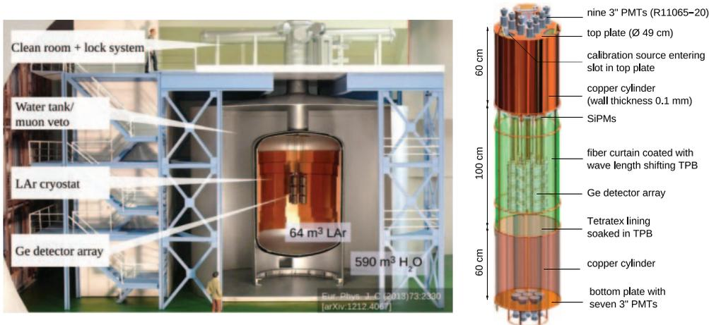
Fig. 1. – Left: setup of the GERDA experiment [7]. Right: assembly of detector array and LAr veto system [9].
