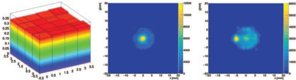
Fig. 4. – Efficiency for the detection of gamma-ray for a single  $4 \times 4$  array (left). Image reconstruction without time-of-flight information: a  $^{22}\text{Na}$  point source in the center (middle), the source displaced by 10 mm (right).
