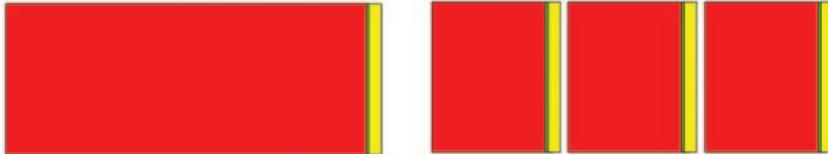
Fig. 6. – The timing error due to the timing spread in the crystal can be reduced by segmenting the gamma-ray detector.
