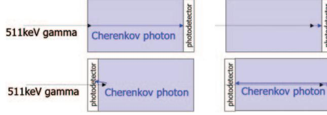
Fig. 5. – The time of arrival of Cherenkov photon depends on their production position and on the position of the photosensor: Cherenkov photons are produced at the entrance (left) and at the exit (right). The photosensor is positioned downstream (above) or upstream (below) of the gamma-ray direction.
