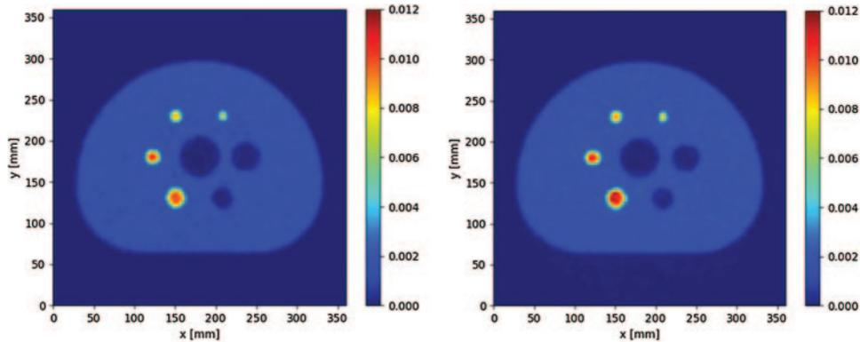
Fig. 7. – Reconstructed images with MLP reconstruction and correction of background attenuation: LSO with CTR 200 ps (left), PbF<sub>2</sub> photosensor TTS 100 ps (right), acquisition time 7.5 s, injected activity of 300 MBq.
