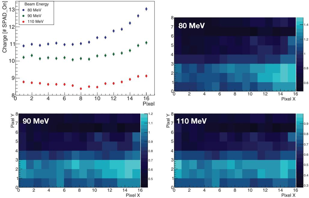
Fig. 5. – Energy released in spad-net sensor from different energies protons. (a) Top left: Charge release in number of detected photon per pixel column. At  $E_p = 80$  MeV there is an increase in the energy release thanks to the Bragg Peak presence; (b)–(d) Top right, bottom left and bottom right: Average energy sensor map. Each square box represent a pixel. The average number of photoelectrons detected are shown with different brightness
