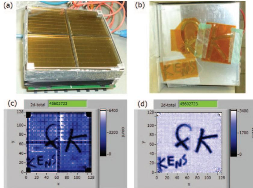
Fig. 3. – (a) 4 H8500 MA-PMTs, (b) Cd “f K KENS” characters, (c) 2D graph of  $128 \times 128$  pixels, (d) corresponding 2D graph of  $128 \times 128$  pixels compensated by the data without the Cd characters.
