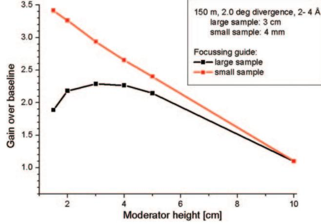
Fig. 5. – Gain in neutron flux on the sample as a function of the height of a cylindrical para- $H_2$  moderator, illuminating a 150 m long focusing neutron guide for beam delivery. The gain factor is given compared to the conventional height of 12 cm. The difference between the two curves is due to the variation of the beam delivery efficiency  $\eta$  with the vertical dimension of the sample.
