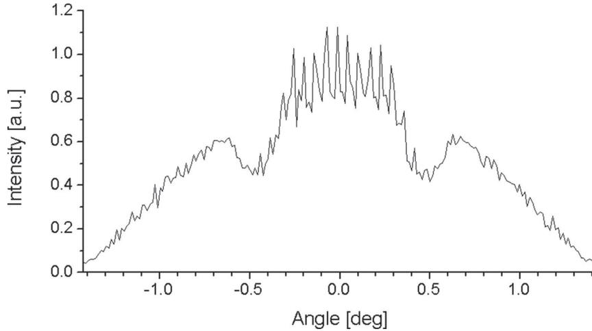
Fig. 1. – Angular distribution of the neutron beam divergence in the vertical direction at the exit of a conventional neutron guide of 8 cm height at its entrance, facing a 10 cm high conventional size neutron moderator. The fine structure in the distribution is inherent to common guide construction routine and in practice only impacts as inhomogeneity the transmission efficiency  $\eta$  of the guide system, without visible effect on the angular resolution.
