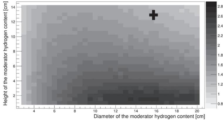
Fig. 2. – Unperturbed cold neutron emission brightness on the side surface of a cylinder shaped liquid para- $H_2$  moderator as function of its height and diameter. The highest brightness corresponds to a flat “pancake” like shape. The black cross indicates a size and shape corresponding to traditional practice.
