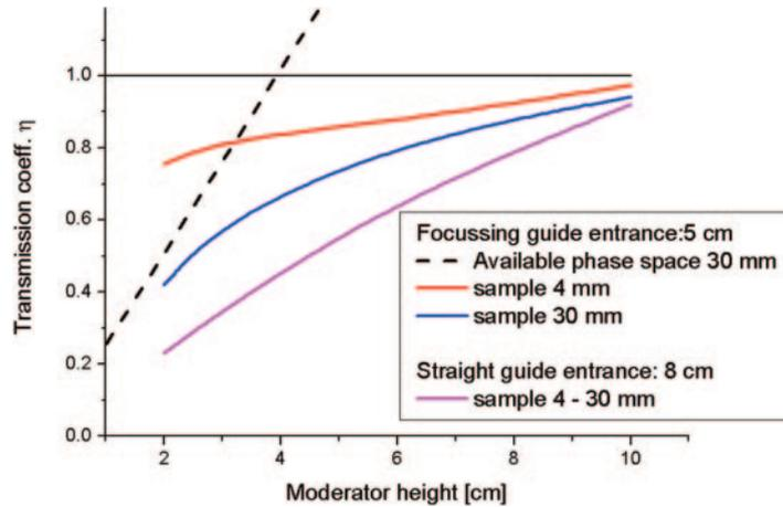
Fig. 4. – Simulated beam transport efficiency  $\eta < 1$  for various neutron guide systems with various sample area dimensions. The dashed line represents an additional theoretical upper limit to the blue curve, derived from phase space volume considerations, as explained in more detail in the text.
