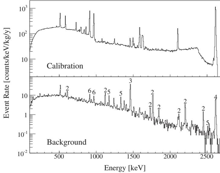
Fig. 2. – Top panel: CUORE-0 calibration spectrum. Bottom panel: CUORE-0 background spectrum; the labels in the plot correspond to identified radioactive peaks:  $e^+e^-$  annihilation (1),  $^{214}\text{Bi}$  (2),  $^{40}\text{K}$  (3),  $^{208}\text{Tl}$  (4),  $^{60}\text{Co}$  (5) and  $^{228}\text{Ac}$  (6). Figure reprinted from [13].
