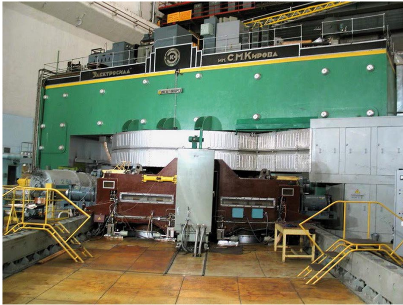
Fig. 3. – Dubna Synchro-cyclotron, initially 460 MeV, later 680 MeV.
